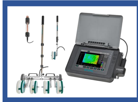
Advanced half-cell Measuring
